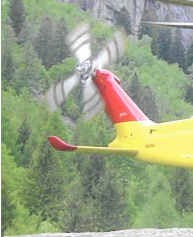
Picture 18 - The tail rotor can be invisible
