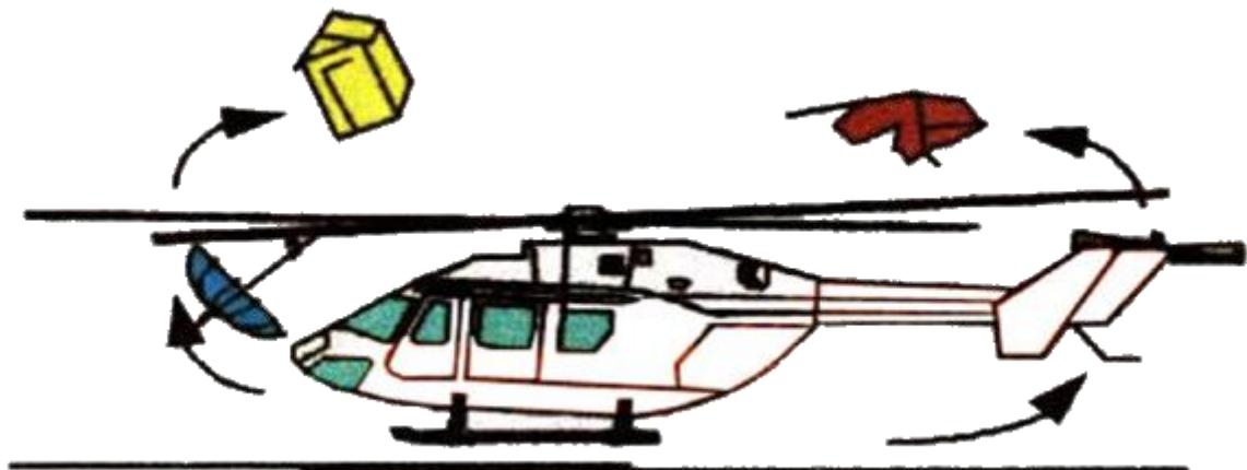
Figure 2 - Rotor downwash can rise several loose material
