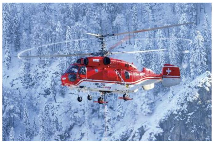
The increase of altitude performance will be implemented as on account of the engine replacement, so that of the currently used auxiliary power unit (APU) for more advanced APU TA-14.
