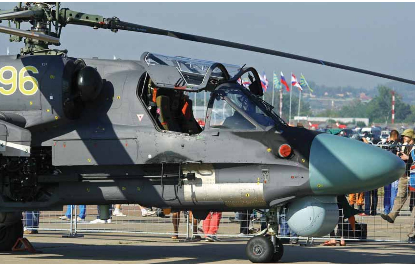
The cockpit of the 'Alligator' is fully armoured, and the fuel system is protected from explosion or fire
