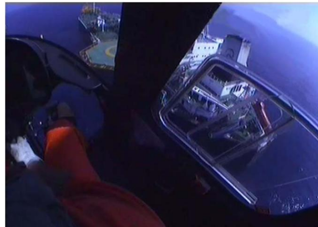
Figure 2I-8 Descending Approach Landing On Helideck - View RH Seat at LDP (15 kts, 50ft ALS, 200 fpm ROD)
