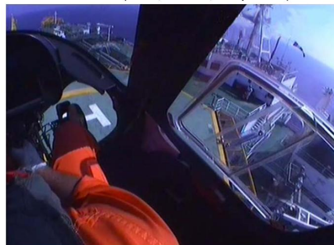
Figure 2I-9 Descending Approach Landing On Helideck - View RH after LDP descending to landing point
