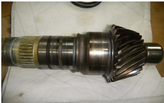
High speed (21,000 rpm) Input Pinion
