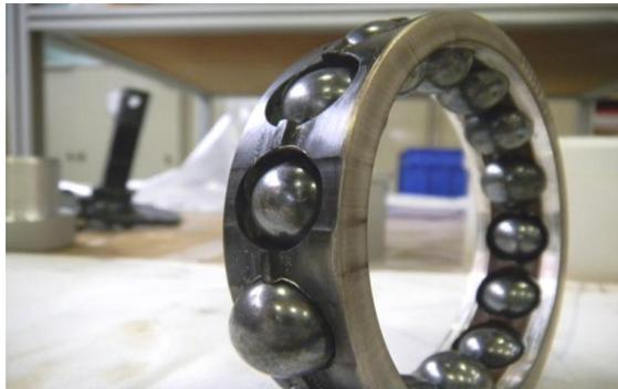
High speed (21,000 rpm) Input Ball Bearing
